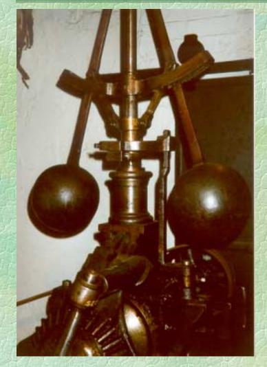
This flyball governor is in the same cotton factory in Manchester. However, this particular governor was used to regulate the speed of a water wheel driven by the flow of the river. The governor is quite large as can be gauged by the outline of the door frame behind the governor.
