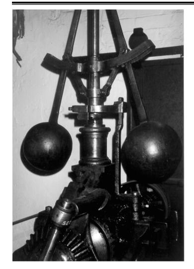
This flyball governor is in the same cotton factory in Manchester. However, this particular governor was used to regulate the speed of a water wheel driven by the flow of the river. The governor is quite large as can be gauged by the outline of the door frame behind the governor.
