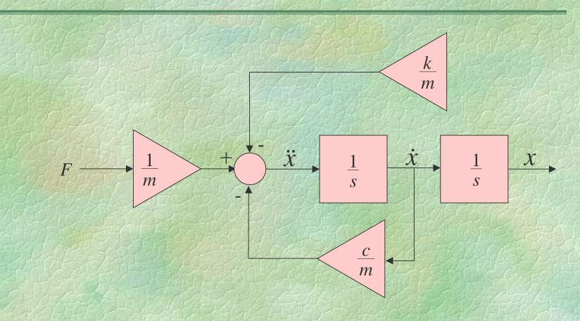
Figure 6(a) represents the same system in transfer function form. The transfer function representation is more compact, and it is useful in understanding the system dynamics. Chapter 4
