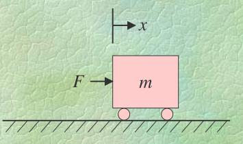
(Note that we use the notation  $\dot{x}$  to represent the time derivatives; thus  $\ddot{x}$  is equivalent to  $d^2x/dt^2$ .) This system may be represented by the block diagram shown in Figure 2. We can expand this block diagram to compute the cart position. In Figure 3 we have added two integrators. The first computes the cart velocity, while the second computes displacement.
