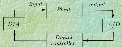
The objective is to cause the output shaft position,  $y(t)$ , to follow a given reference signal,  $y^*(t)$ .
